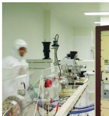
The third accelerator located at this node is a Colutron low energy ion implanter (0.01-15keV) predominantly used for phosphorus implantation of quantum devices (Figure 3). It was originally commissioned in 2001 and is equipped with a: G2 ion gun, beam imaging system, computer controlled ion selection, beam scanning for large area implantation, beam on demand and single ion detection capabilities.
