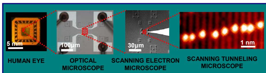
Figure 1: Range of technologies and length scales that have been aligned compatibly from optical to scanning electron to scanning tunnelling microscopes. Our unique registration technique bridges the gap between the atomic and micron length scale.
