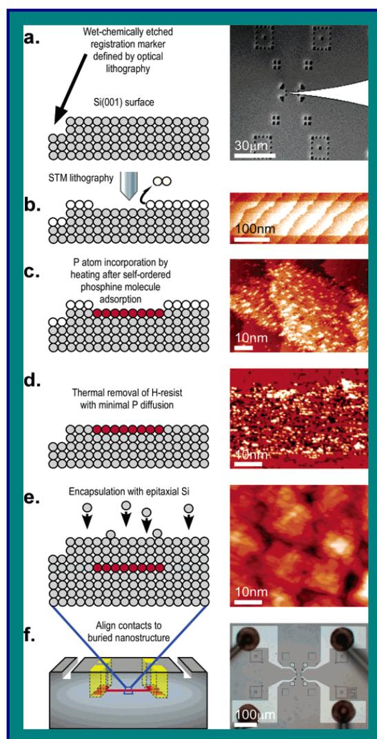
Figure 2: Device fabrication strategy for the creation of Si:P atomic devices using scanning probe microscopy.
