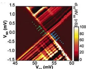
**FIGURE 6** A close-up of one of the Coulomb blockade transitions for a 7 donor dot showing a dense spectrum of excited states.
