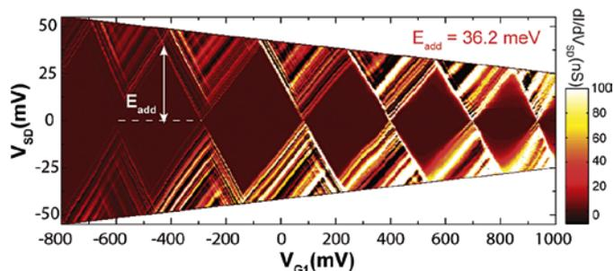
**FIGURE 5** The stability diagram for a 7 donor dot showing a dense spectrum of excited states.
