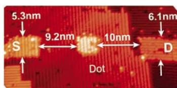
**FIGURE 4:** STM lithography showing a  $4.6 \times 4.6 \text{ nm}$  desorbed area which will incorporate 7 P donors.
