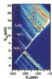
**FIGURE 7:** The stability diagram for a single donor dot showing an addition energy of  $42 \pm 2 \text{ meV}$  and lines at the excited state energies of 11 and 13 meV. Additional lines observed are due to the one dimensional subbands of the lead geometry.
