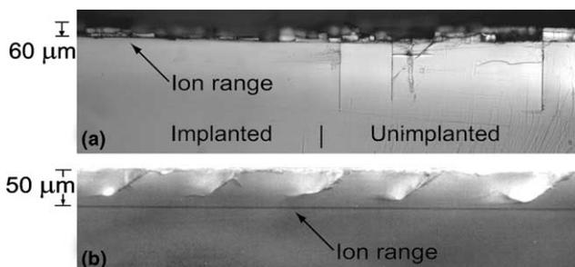
Fig. 1. (a) Fracture pattern profile of MgO crystal in the implanted (left) and unimplanted (right) regions and (b) fracture pattern profile in the implanted sapphire crystal.
