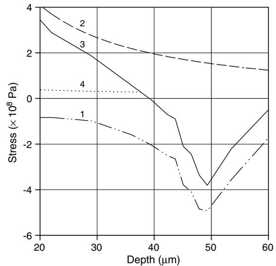
Fig. 2. Distribution of stress with depth in the implanted sapphire, 1 – implantation-induced stress, 2 – thermal stress, 3 – net stress, 4 – stress required for crack propagation.
