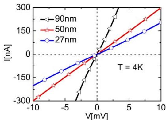
Figure 2: Four-terminal I-V characteristics of 90 nm (triangles), 50 nm (stars) and 27 nm (circles) wide P:Si wires at 4 K showing ohmic conduction with low resistivities down to  $1 \times 10^{-8} \Omega\text{cm}$ .
