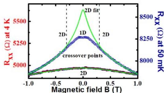
Figure 3: Crossover from 2D to 1D weak localisation is observed in the magneto-transport of a 90 nm wide Si:P quantum wire when lowering the bath temperature from 4K to 50mK. Comparison with fits to 2D weak localisation theory (green lines) allows us to calculate the electrical width of the wire, which is found to be equal to the STM defined lithographic width.
