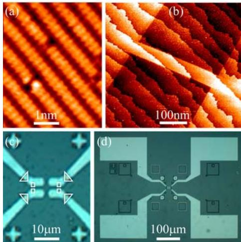
Figure 1: STM images of (a) the hydrogen-terminated Si surface demonstrating atomic-resolution and (b) a 50 nm × 310 nm wire pattern using STM lithography. Optical microscope images of (c) the central contact area showing overlap between the registration markers and the ohmic metal and (d) the entire device.
