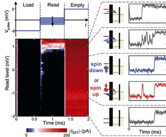
**FIGURE 3** Three-level pulse sequence for single-shot spin readout. The main panel shows averaged SET current as a function of the “read” pulse voltage. The time-resolved single-shot traces highlight the correct tuning region where projective readout of spin-down (blue) or spin-up (red) electrons is obtained.
