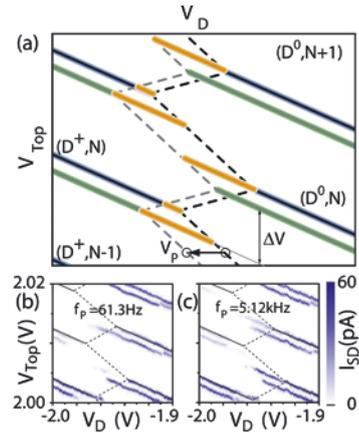
**FIGURE 1** Sketch (a) and measurement (b,c) of the SET current while pulsing the donor gate in a qubit structure. The frequency dependence of the non-equilibrium currents (orange lines in (a)) allows the extraction of the electron tunnel rate between donor and SET island.
