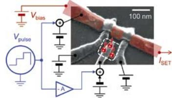
**FIGURE 2** Circuit diagram and SEM image of the qubit device employed for single-shot spin readout.
