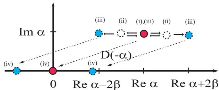
**Figure 4.** Schematic diagram showing the phase space evolution of the bus amplitudes corresponding to the various qubit computational basis states. The labels (i)–(iv) correspond to the evolution stages, as shown in the circuit diagram in figure 3.
