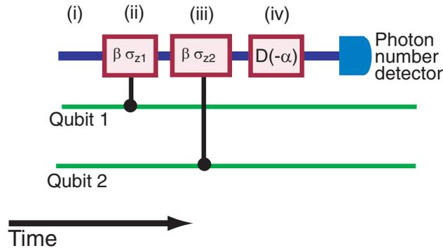
**Figure 3.** Circuit diagram for a two-qubit parity gate based on controlled displacements between the qubits and the ‘probe’ bus, followed by bus measurement.
