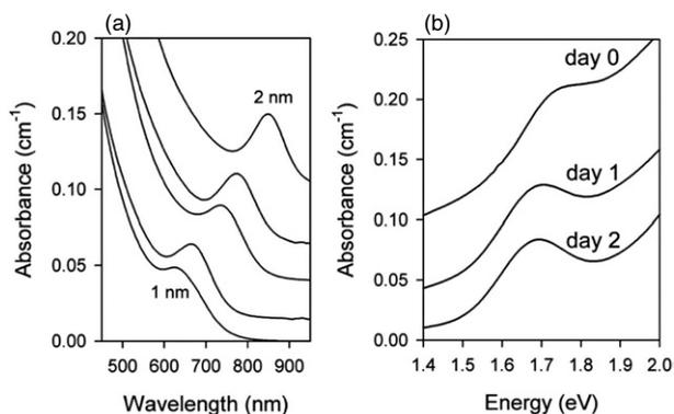
**Figure 1.** (a) Absorption spectra from a range of PbS NC solutions demonstrating that tuning of the first exciton peak throughout the strong quantum confinement regime can be achieved. (b) Natural size focusing of a PbS NC solution in hexane when stored in the dark at room temperature for two days. An absolute absorbance scale is used for direct comparison, revealing the dramatic reduction in the infrared tail that occurs with the size focusing.
