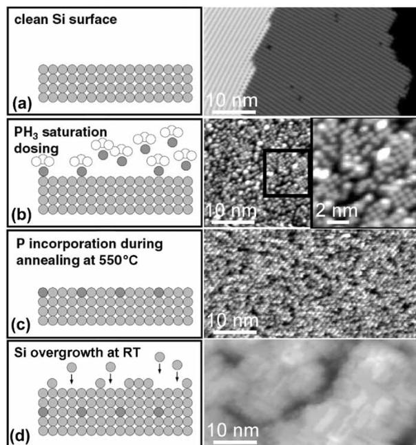
Figure 5. Schematics and STM images describing the sample preparation process for the fabrication of a phosphorus in silicon  $\delta$ -doped layer used for SIMS analysis to determine segregation lengths and magnetoresistance measurements to determine the degree of electrical activation.
