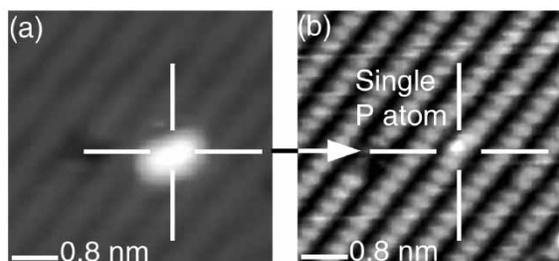
Figure 4. STM images of atomically controlled single P atom incorporation into Si(100). (a) hydrogen terminated Si(100) with a  $\sim 1$  nm diameter hydrogen desorption point. (b) the same area after  $\text{PH}_3$  dosing and annealing to  $350^\circ\text{C}$  showing a single P atom incorporated at the location defined by the hydrogen desorption point.
